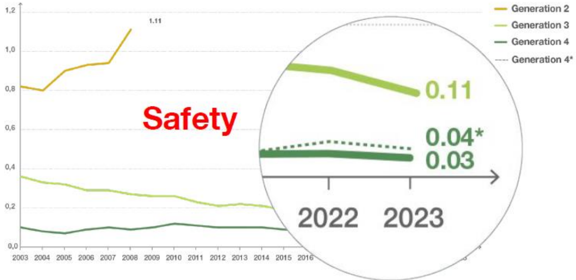
10 year moving average fatal accident rate (per million flights) per aircraft generation
